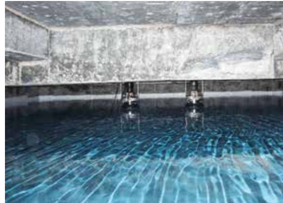
Figure 2: The China-Japan collaboration placed new water Cherenkov-type muon detectors under the existing air-shower array in 2014. (Image by IHEP)
