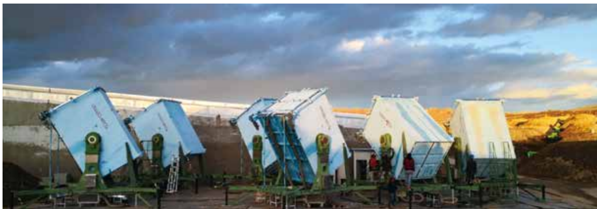
The telescopes in the Wide-Field-of-View Cherenkov Telescope Array (WFCTA). Each of them can be tuned 0–90 degrees in elevation to effectively target on the goals. (Credit: IHEP)
