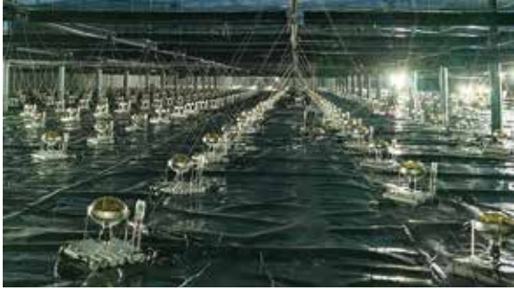
Inside the WCDA's pond #3 with the PMT array installed in July 2020 before water filling
