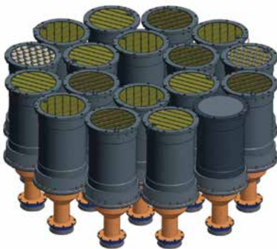
(Left) Modules of the high-energy (HE) detector aboard Insight-HXMT and (Right) the corresponding fields of view (FOVs) of HE in combination with those of other two detectors aboard Insight-HXMT , the medium-energy (ME) and low-energy (LE) ones. The differently oriented FOVs commonly constrain and hence determine the localization of the target. (Credit: IHEP)
