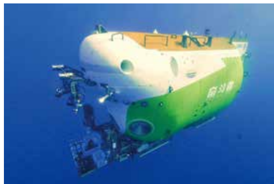
Fendouzhe , also known as Striver in English, the submersible that has set a national record by diving to a depth of 10,909 meters in the Mariana Trench. [Photo/China Daily]
