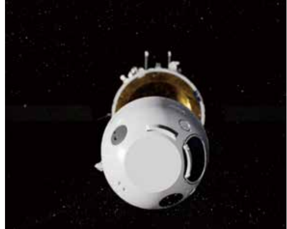
Illustration of CE-5 returner detaching from the orbiter (Computer animation by CASC)
