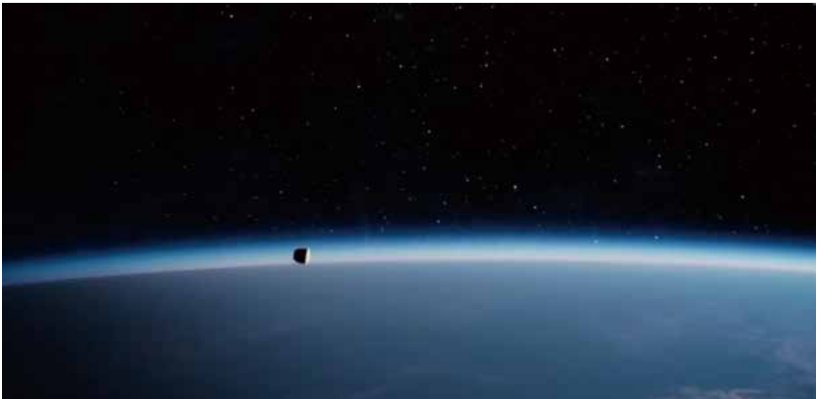
Computer simulation of the big “dap” of CE-5, a bounce back to outer space after the first entry into the Earth atmosphere. This smart maneuver aims to consume extra kinetic energy and slow down to an acceptable speed for a second entry, so as to avoid being burnt out by the excessive heat produced by the friction between the overspeed capsule and the air. (Animation by CASC)
