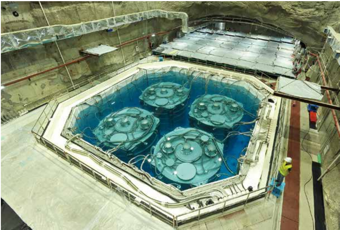
Antineutrino detectors are submerged in water pools at the site of the Daya Bay experiment in Guangdong, China. (Image by IHEP)
