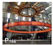
The world's first nuclear power stainless steel giant ring (15.6 m in diameter) in one piece was manufactured by a new forging technology developed by researchers from the CAS Institute of Metal Research (IMR).
