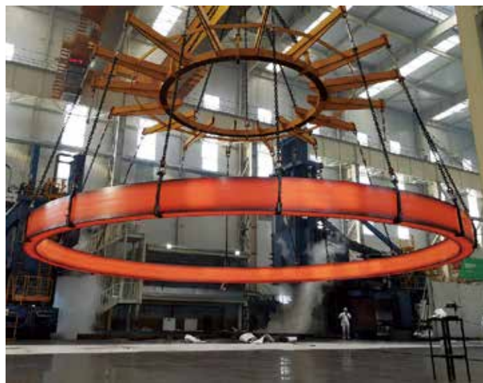
The world's first nuclear power stainless steel giant ring (15.6 m in diameter) in one piece was manufactured by additive forging technology. (Image by SUN's Lab)
