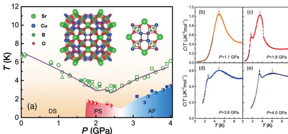
Fig. 1 (a) Phase diagram of  $\text{SrCu}_2(\text{BO}_3)_2$  (crystal structure in the inset) from high pressure  $C(T)$  measurements. Examples of  $C(T)/T$  curves are given in (b)–(e), where the orange arrows indicate the hump location.
