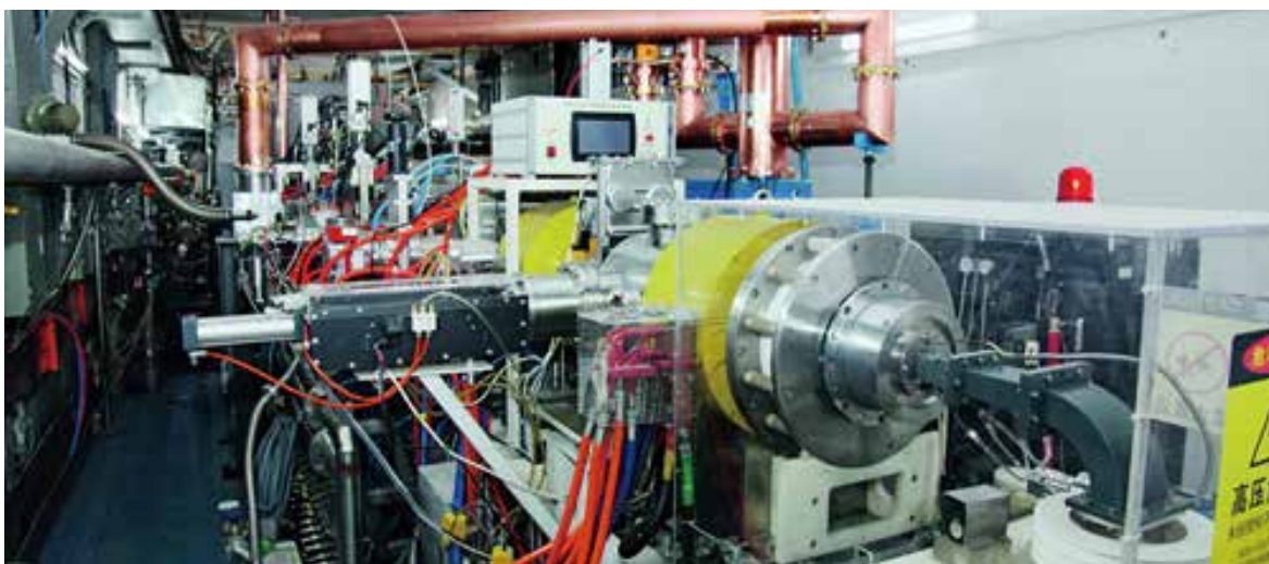
The “starting gun” of ADS: the superconductive proton linear accelerator that feeds the system with ion sources (Credit: IMP)
