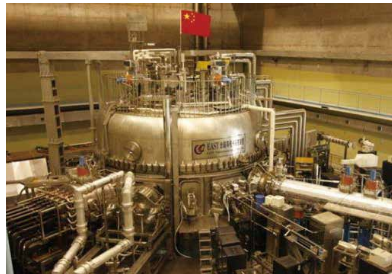
China's Experimental Advanced Superconducting Tokamak (EAST), a nuclear fusion experimental device in Hefei, China. (Credit: CASHIPS)
