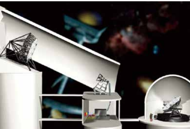
LAMOST consists of a reflecting Schmidt corrector M_A (low right in the picture) at the northern end, a spherical primary mirror M_B (upper left in the picture) at the southern end and a focal plane in between. Both the primary mirror and the focal plane are fixed on their ground bases, while the reflecting corrector is left free to track the motion of celestial objects. A total of 4,000 optical fibers are installed on the focal plane in between, being connected to 32 CCD detectors. During an observation, the fibers transmit the starlight focused on them to the spectrographs beneath the focal plate, where the starlight is decomposed into spectra. (Credit: NAOC)
