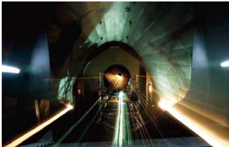
Light beams glitter inside the huge tube of LAMOST. This mammoth astronomical telescope represents the most challenging application of active optics so far, having achieved both an extremely large field of view (5 degree) and a big aperture (7.8m). (Credit: NAOC)
