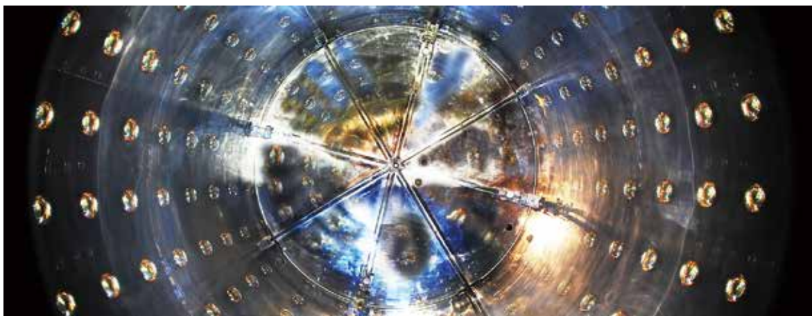
The neutrino detector immersed in water at the Daya Bay Neutrino Experiment (Image: IHEP)
