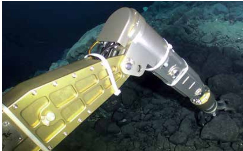
SeaStar 6000 collecting rock samples from sea bottom (Credit: SIA)
