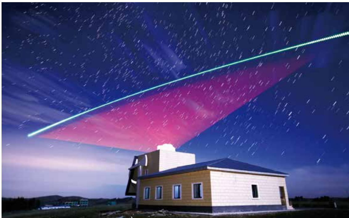
Shown here is a time-lapse exposure (10 to 15 seconds) image taken by the team during the satellite's passing over the Nanshan optical ground station (OGS). The green line is the bacon laser from the satellite to the ground, and the red light the bacon laser from the ground station to the satellite. (Photo by ZHU Jin)
