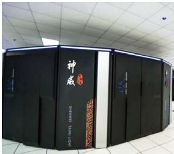
With a Linpack mark of 93 petaflops, Sunway TaihuLight developed by the National Supercomputing Center in Wuxi became the world’s fastest supercomputer in June 2016.
