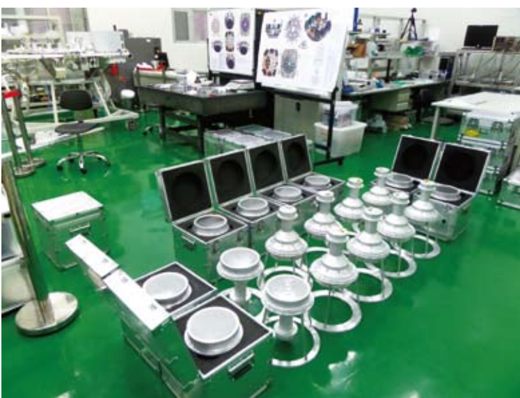
The 18 HXMT/HE main detectors that will be onboard HXMT. (IHEP, November 2015)
