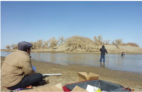
Researchers conducting an in situ measurement of hydraulic conductivity of the Lower Heihe River bed.
