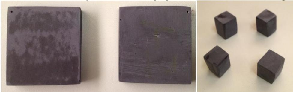
*Fig. 3 – The new molded samples of epoxy resin composite structure*
