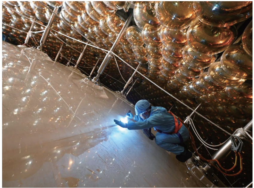
Seen here is a patch of the acrylic sphere (bottom) of the central detector, and the surrounding photomultiplier tubes (the yellow, bubble-like “small balls”). Filling the acrylic sphere of a record size, the volume of the liquid scintillator is 20 times larger than the previously largest one in the world. (Credit: JUNO Collaboration)
