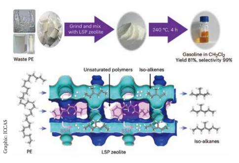
Turning plastic bags or waste polyethylene (PE) into premium gasoline using earth-abundant layered selfpillared (LSP) zeolite catalysts.
