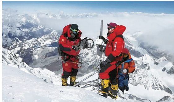
Setting up the world's highest weather station at the altitude of 8,800 meters.
