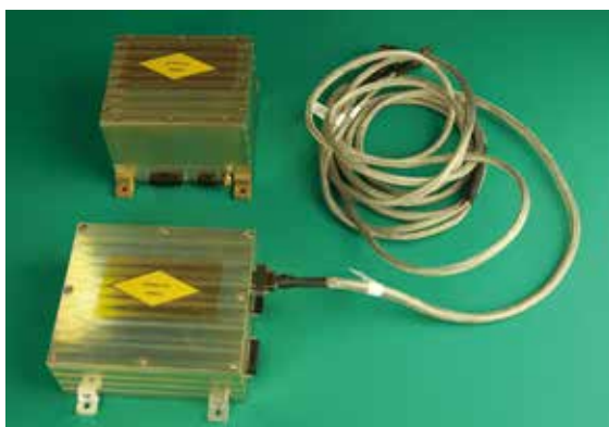
The Lunar Lander Neutrons & Dosimetry (LND) aboard Chang'e-4 developed by Germany.
