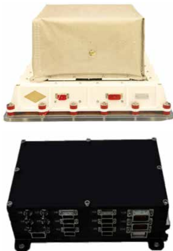
POLAR photos. Upper: Gamma-ray burst detector (OBOX); Bottom: Electrical cabinet (IBOX). (Image by IHEP)
