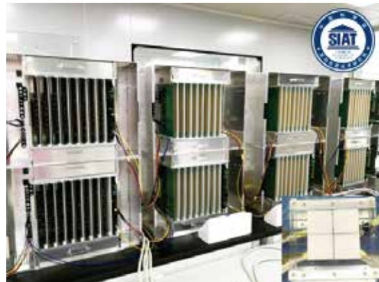
Large scale (thousands of channels) ultrasound transducer and system specifically for ultrasound neuromodulation.
