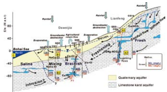
Cross section showing the conceptual hydrogeological and hydrogeochemical model derived from hydrological, geochemical and isotope data. Arrows in aquifers indicate groundwater flow direction. (Image by HAN Dongmei)
