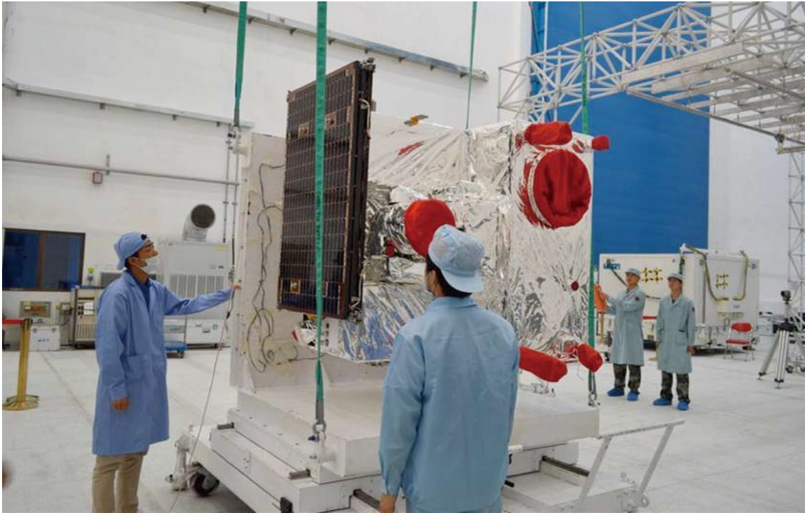
Shot on July 27, 2016, the photo shows technical staff installing the solar wing for the experimental quantum communication satellite at the Jiuquan Satellite Launch Center in Jiuquan, northwest China's Gansu Province. (Photo: Xinhua)
