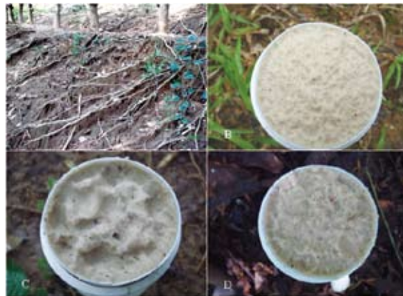
Serious splash erosion in the riser bank under rubber plantation (A), and splash potential under open field (B), rubber plantation (C) and tropical rainforest (D).
