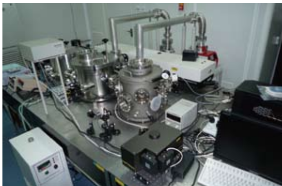
The DUV laser photochemical reaction apparatus developed by the Technical Institute of Physics and Chemistry.
