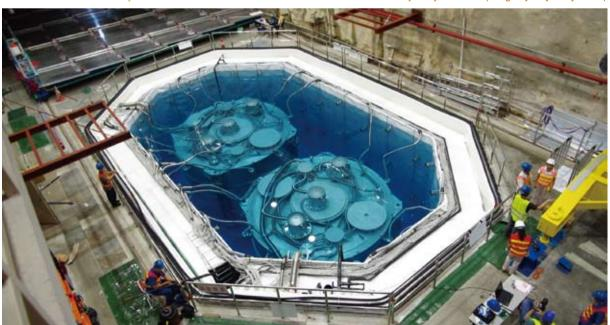
Daya Bay Experiment consists of eight 110-ton antineutrino detectors, immersed in water pools in three experimental halls, to detect antineutrinos from the nearby reactors. Shown here are two antineutrino detectors in the Daya Bay near hall. (Image by Daya Bay Team)
