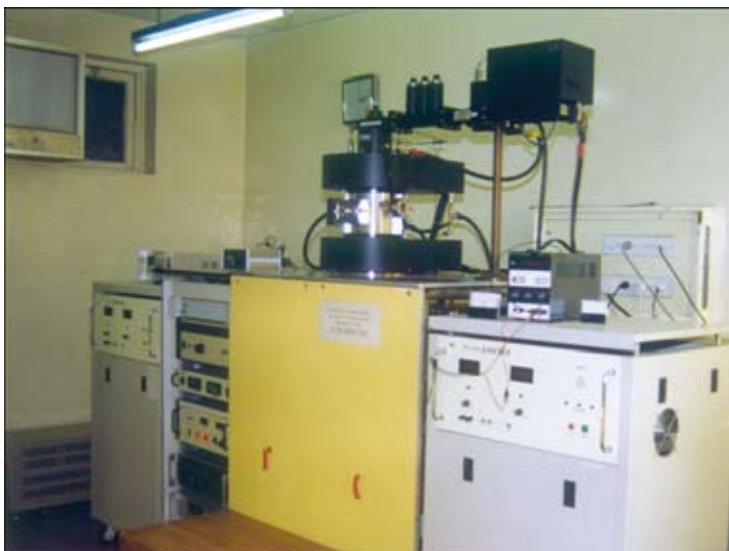
Figure 1: Microwave plasma enhanced chemical vapor deposition system developed by the team for the involved experiments.
