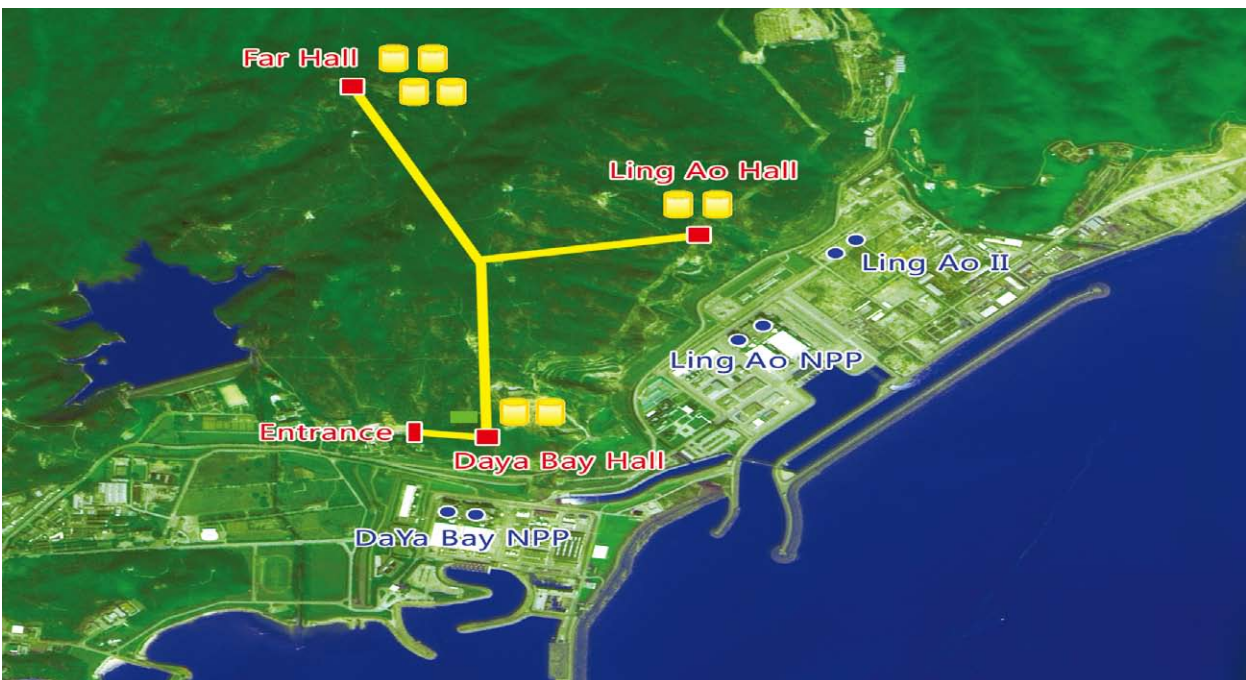
A pair of antineutrino detectors is positioned respectively in Daya Bay Hall (EH1) and Ling Ao Hall (EH2), while another set of four is positioned in the Far Hall (EH3) almost two kilometers away.
