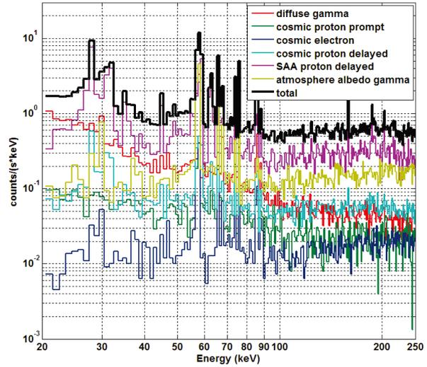
Fig.3 The simulated in-orbit background induced by various components at the time 10 minutes from the Southeastern Atlantic Anomaly (SAA) region and 100 days after launch.
