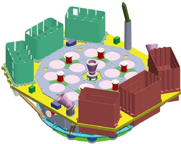
Fig.2 The payload assembly of HXMT. The 18 cylindric detector units of HE are in the center of the assembly and are covered by veto plates. The three cyan detector boxes in the upper left belong to LE, and the three brown boxes in the lower right represent ME. On the payload assembly there are three star trackers, three charged particle monitors, and an antenna.
